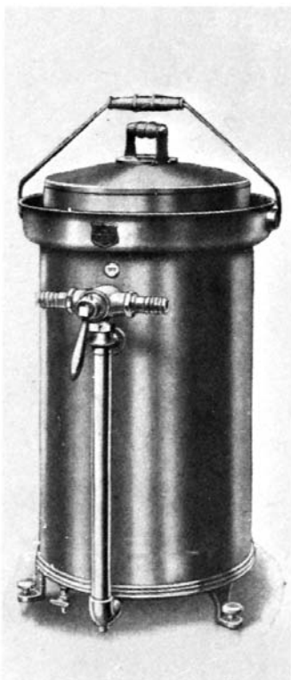
FIG. 1 Stillman-Type Portable Cubic-Foot Standard
